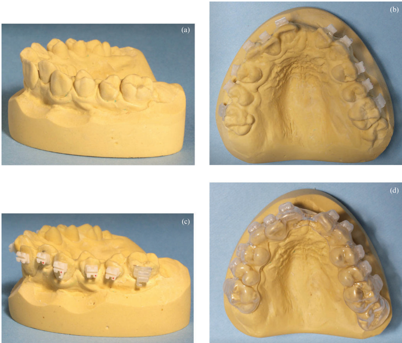
Figure 3 Brilliant brackets on the study models. (a) Upper arch prior to fixed appliance; (b) Aesthetic brackets applied to upper model including molars; (c) Aesthetic brackets applied to upper model; (d) Occlusal splint with aesthetic brackets embedded prior to test MRI
